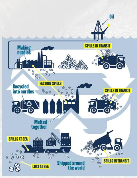
Plastic pellets can be spilled at any point of handling in the plastics supply chain, including production, transport, processing and even plastics recycling.
